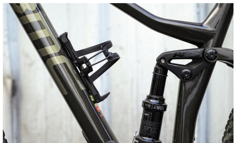
▲Nuvo's new side bottle cage with recycled plastic, PA66+40% with GRS Certification, weights 48g.
