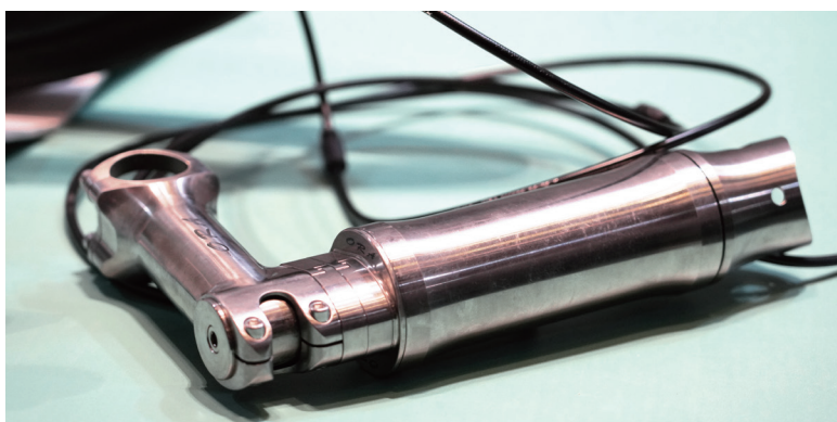
▲Titanium internal routing stem.
